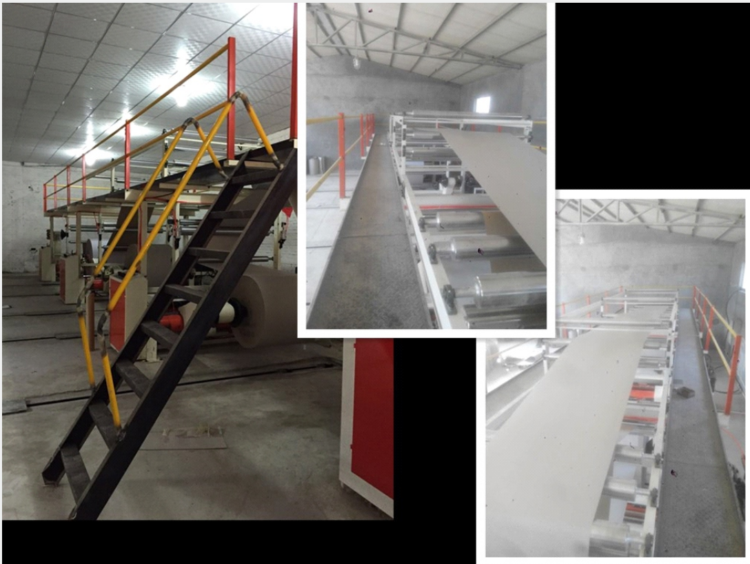
( 4Bracket ) 1 set of Overpass Conveyor Device
