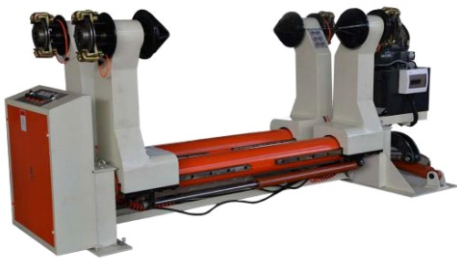
3SETS OF SYZ HYDRAULIC SHAFTLESS MILL ROLL STAND
